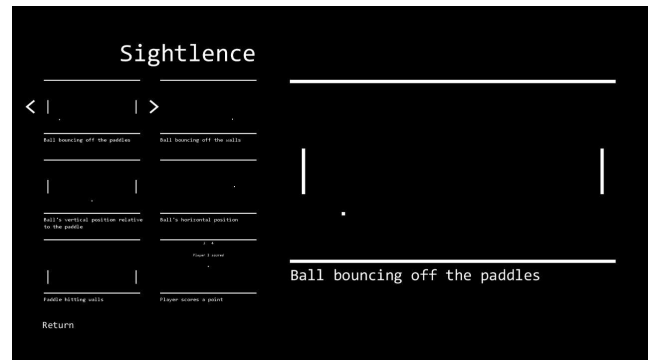
Figure 2: The tutorial in Sightlence provides isolated output of each individual haptic signal for learning purposes.
